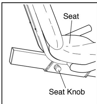
**the console when you pedal.** To adjust the seat, first turn the seat knob counterclockwise two or three turns to loosen it (if the seat knob is not loosened enough,
