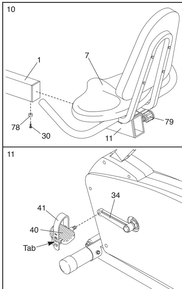
11. Identify the Left Pedal (40) (there is an "L" on the Left Pedal for identification). Using an adjustable wrench, tighten the Left Pedal counterclockwise into the left Crank Arm (34).
