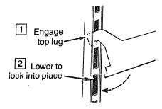
To replace shelves: Select desired shelf height. With shelf front raised slightly, engage top lugs in tracks at rear of cabinet. Then lower front of shelf until it locks into position.
