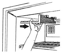
To remove shelf, pull it away from cabinet wall to disengage pins on shelf from holes in wall.
