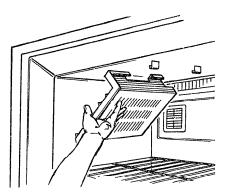
Then tilt shelf to disengage it from supports at top of freezer compartment, and take shelf out.
