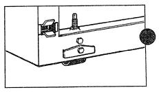
Turn roller adjusting screws clockwise to raise the refrigerator, counterclockwise to lower it. Use adjustable wrench (3/8" hex head bolt) or pliers.
