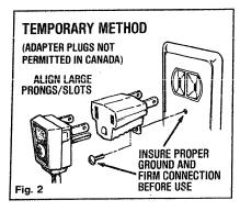
The larger slot in the adapter must be aligned with the larger slot in the wall outlet to provide proper polarity in the connection of the power cord.
