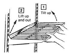
To remove shelves: Tilt shelf up at front, then lift it up and out of the track on rear wall of refrigerator.
