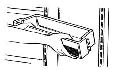
To remove: Lift Porta-Bin straight up until mounting hooks disengage.
