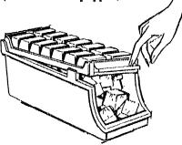
Ice trays are designed to release cubes easily into a companion ice storage bin. Just invert tray, insert one end into slot at rear of bin, press at front right side, and cubes will drop into bin.
