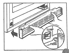
To replace base grille, align prongs on back of grille with clamps in cabinet and push forward until the grille snaps into place.
