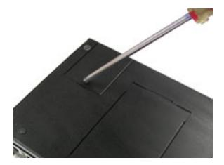
Step 1. Unscrew a screw and take off the chassis cover as indicated.
