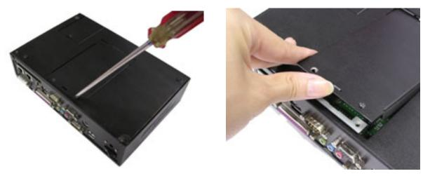
Step 1. Unscrew two screws as indicated and take off the chassis cover.
