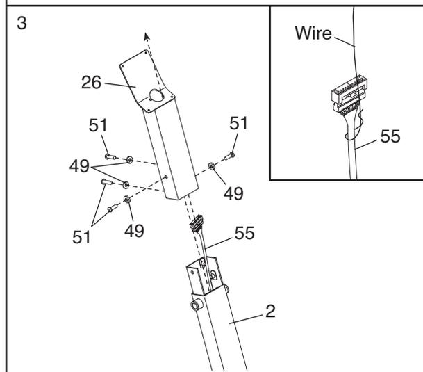
Insert the Console Bracket (26) into the Upright (2). **Be careful to avoid pinching the Upper Wire Harness (55).** Attach the Console Bracket with four M8 x 25mm Button Screws (51) and four M8 Split Washers (49).
