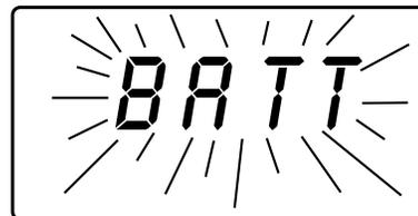
**NOTE:** The thermostat will still keep the current time and your programs in memory until new batteries are installed. After confirming new batteries have been inserted, the thermostat will return to normal operation.
