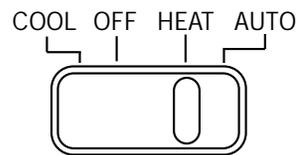
■ Slide System Selector Switch to HEAT or COOL to program the corresponding system.
