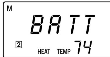
**NOTE:** The backlight will not operate in low battery condition. Replace with 2 new AA alkaline batteries to restore the Backlight function.
