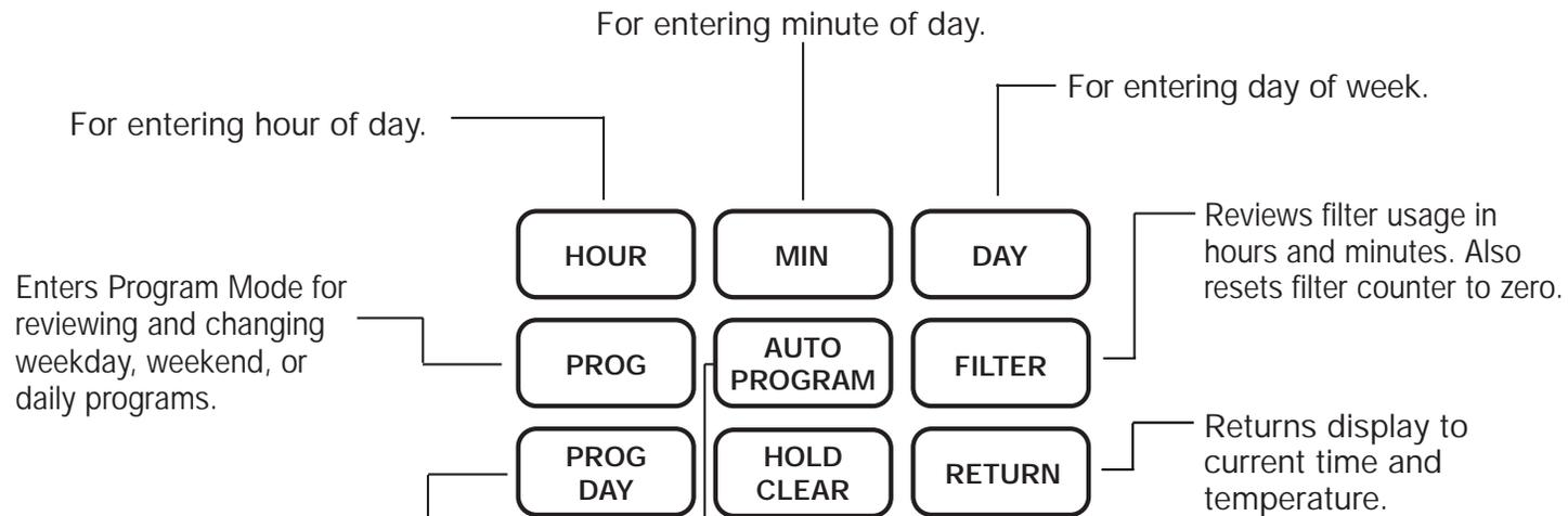
Automatically programs the thermostat to its built-in ENERGY STAR<sup>®</sup> compliant program settings. See page 17.
