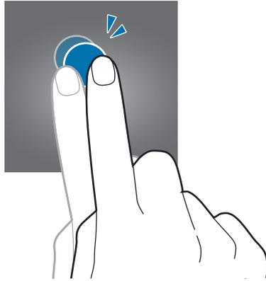
To check the current status of the Gear and view the remaining battery power, double-tap anywhere on the screen with two fingers. You can also adjust the volume and the brightness of the display.
