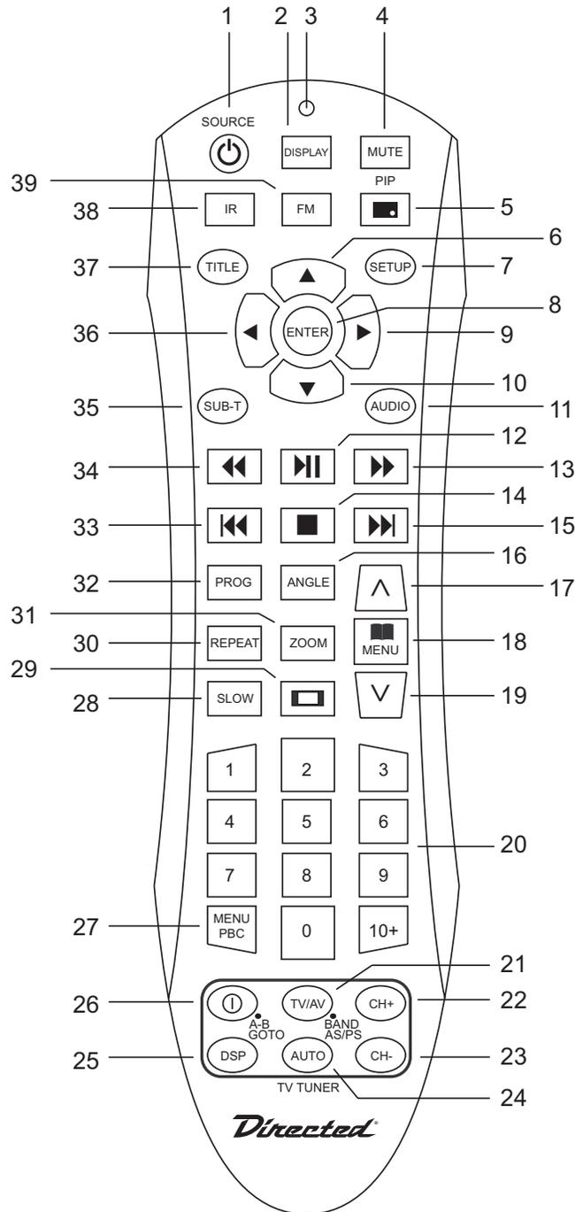
1. POWER and video SOURCE button: Press and hold to turn the unit ON or OFF. When the unit is on, press SOURCE button to change the mode.
