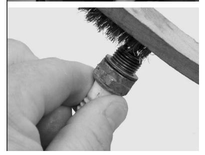
B Gap if necessary to 0.02" (0.5 mm).
