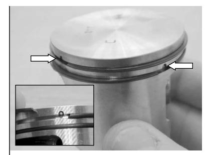
13.15 Install one wrist pin retaining clip.
