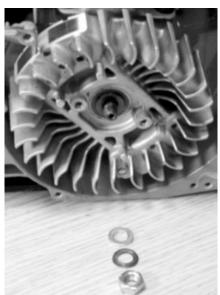
16.3 Screw on flywheel removal tool finger tight. Unscrew tool 1 ½ turns leaving approximately 1/8 inch (5 mm) space between tool and flywheel.
