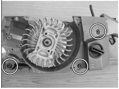
19.3 Separate crankcase and fuel tank.
