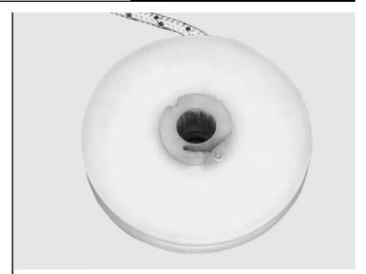
8.11 Install starter rope and tie knot.
