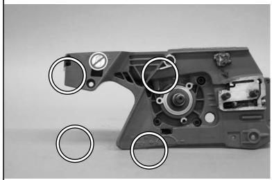
20.3 Heat the flywheel side crankcase with heat gun for 5 minutes, approximately 150° F (65.5° C).
