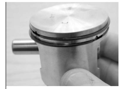
13.18 Align piston in correct orientation.
