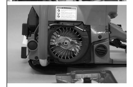
This section covers the removal, inspection, and installation of the flywheel. Removal of the starter and spark plug is required. Refer to sections 6 and 8 if necessary.
