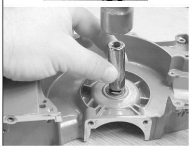
20.6 Heat the clutch side crankcase with heat gun to 150° F (65.5° C).
