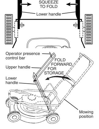
2 POSITION / "ADJUSTABLE" HANDLES When setting you handles up from the storage position, the lower handle will automatically lock into mowing position.
