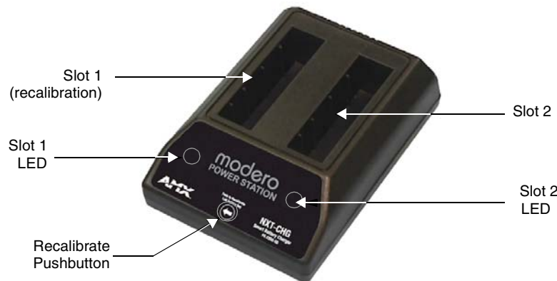
FIG. 31 Component locations on the NXT-CHG
