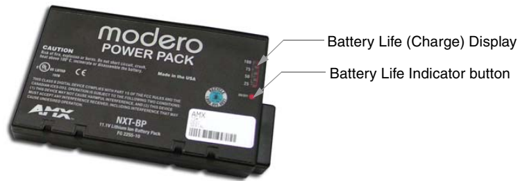
FIG. 26 NXT-BP Battery Pack (showing the battery life indicator and button)
