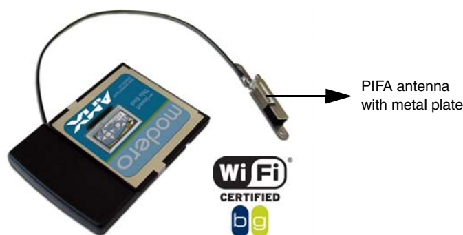
FIG. 15 NXA-WC80211GCF 802.11g wireless card
