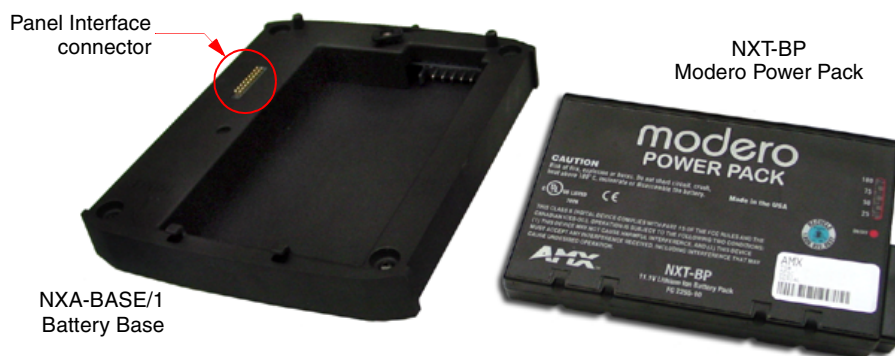
FIG. 25 NXA-BASE/1 Kit (consists of one BASE/1 and a single NXT-BP)
