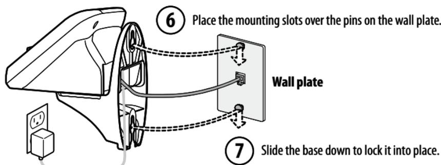
Note: To mount the phone directly on the wall, insert two 1 3/8 inch, #10 screws (not supplied) into the wall using anchors suitable for the wall material. Place the screws 3 15/16 inches apart, and allow 1/8 inch free space between the wall and screw heads.
