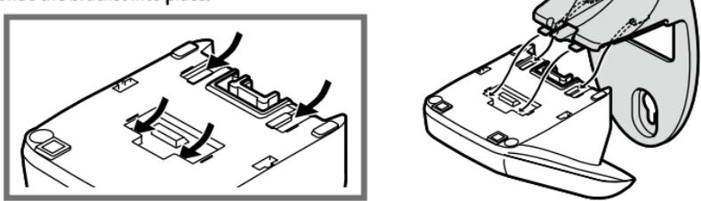
**4** Hook the AC adapter cord into the smaller notch at the bottom of the bracket, and let the cord hang below the bracket.
