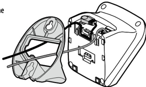
**3** Line up the four tabs on the wall mount bracket (two at the top and two at the bottom) with the four notches on the bottom of the base. Slide the bracket into place.
