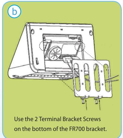
Align the FaceIN terminal with the pins on the mounting-plate and secure the two together with the 2 Phillips head screws. Be careful not to pinch the AC cord. When finished, plug the Power Adapter into an AC wall outlet.
