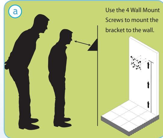
Mount the FaceIN terminal by choosing your "shortest" employee and have them stand in front of the FR700 device. Hold the device on the wall so that this employee can comfortably center their face in the LCD display window. Mark the height of the FR700 on the wall.
