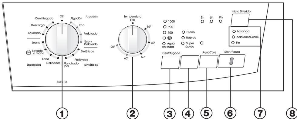
**1** Programme selector dial and On/Off switch**2** Temperature selector**3** Spin reduction button**4** Options button**5** AquaCare button**6** Start/Pause button**7** Programme progress display**8** Delay Start button
