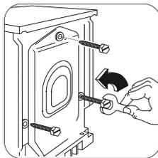
1. Unscrew and remove the three rear screws by means of a key.
