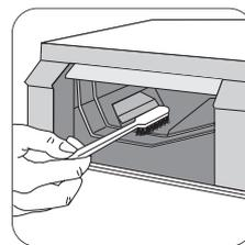
Having removed the drawer, use a small brush to clean the recess, ensuring that all washing powder residue is removed from the upper and lower part of the recess.
