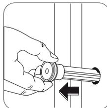
2. Open the porthole and remove the polystyrene block fitted with adhesive tape on the door seal.
