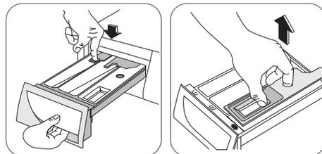
To aid cleaning, the top part of the additive compartment should be removed.
