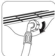
The appliance must be connected to a cold water supply.
