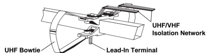
**Note:** Both sections of the UHF/VHF isolation network should remain parallel to the main boom.
