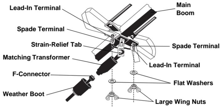
To connect coaxial cable to your antenna:
