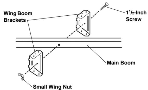
5. Insert the top and bottom wing booms into the wing boom brackets. Secure them with the four supplied 1 1/4-inch screws and small wing nuts, as shown.
