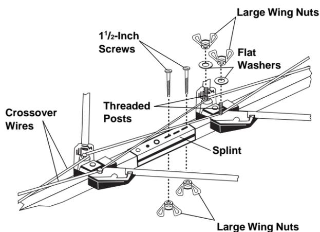
2. Use the supplied hardware to loosely attach one of the supplied mast clamp assemblies to the main boom, as shown.
