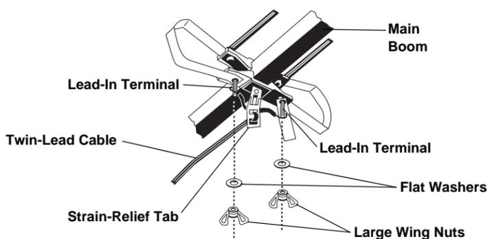
To connect flat, twin-lead cable to your antenna:
