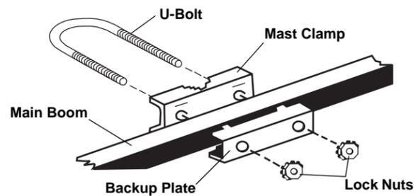
3. Attach the other mast clamp assembly to the cradle boom. (Be sure it faces the same direction as the main boom's mast clamp assembly, shown above.) Fold out the two sets of metal support straps on the cradle boom and attach them to the corresponding holes on the main boom using the two supplied 1 1/2-inch screws and large wing nuts.
