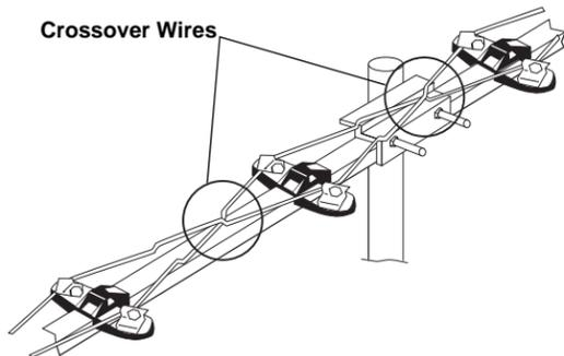
3. Set up the mast, then rotate it so the antenna's shorter elements point toward the broadcast antennas of the stations you want to receive.
