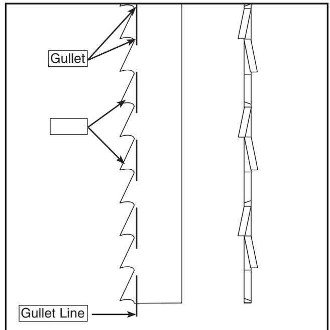
**Figure 9.** A precision tooth, raker set blade.
