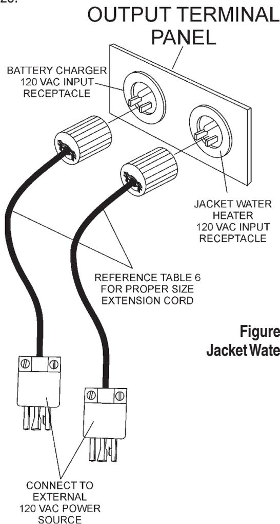
**Figure 56. Battery Charger & Jacket Water Heater Power Connections**
