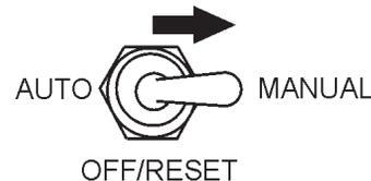
Figure 42. MPEC Control Switch (Manual Position)
