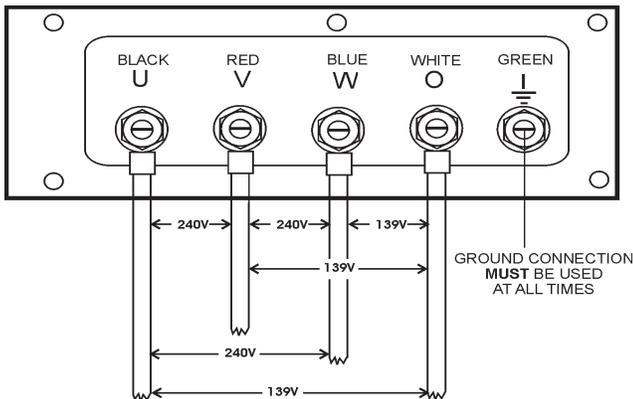
**Figure 23. Output Terminal Lugs 240/139V Three Phase Connections**
