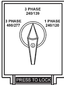
**Figure 22. Voltage Selector Switch 240/139V Three-Phase Position**
