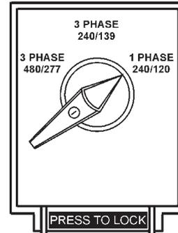
**Figure 29. Voltage Selector Switch 240/120V Single-Phase Position**
