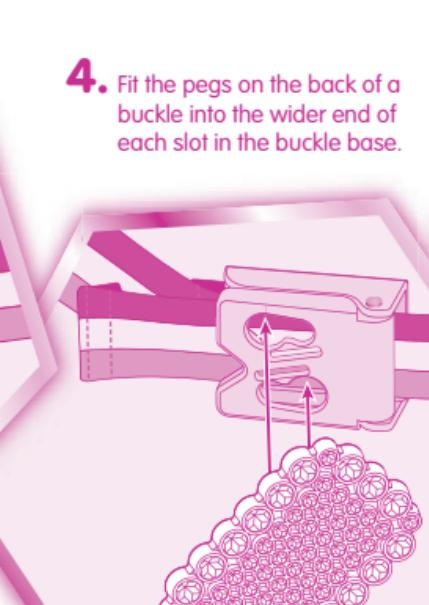
4. Fit the pegs on the back of a buckle into the wider end of each slot in the buckle base.
