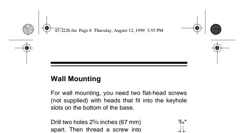
Align the keyhole slots with the mounting screws and slide the station downward to secure it.
