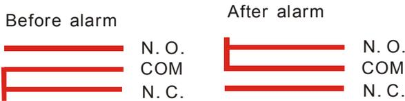
Fig 2.8 Relay Output Status
