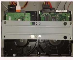
Fig 2.1 Installing hard drive
