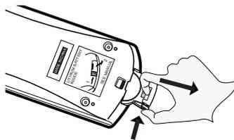
**NOTE:** If the remote does not work properly, remove the battery, wait for a few seconds, replace the battery and try again.
