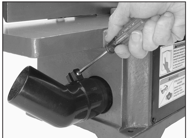
Figure 19. Installing the dust chute.
