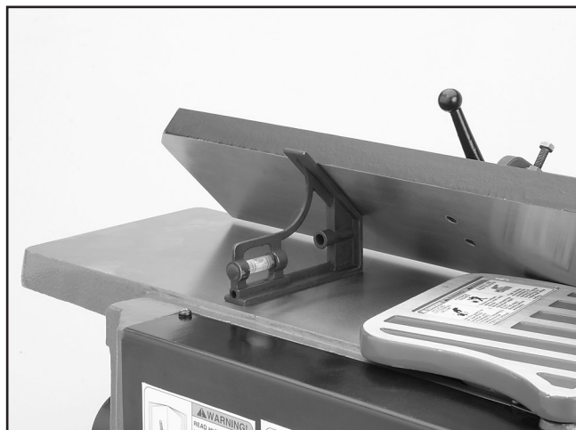
Figure 25. Checking the inward 45° stop.
