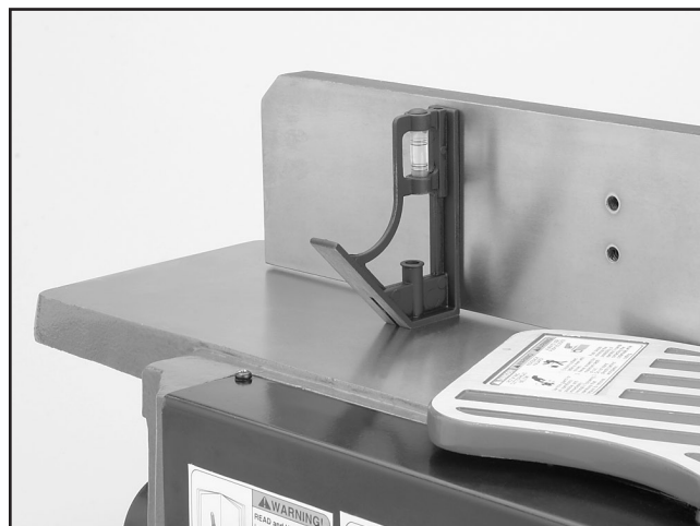
Figure 24. Checking the 90° stop.
