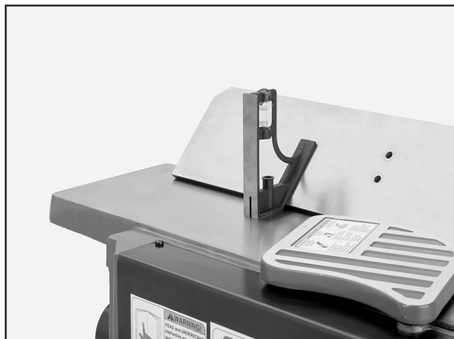
Figure 27. Checking the outward 45° stop.
