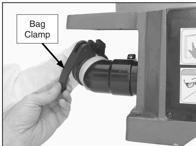
Figure 20. Attaching the dust collection bag.
