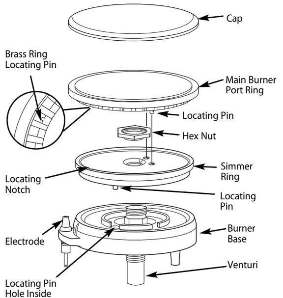
After cleaning, it is important to make sure the Locating Pin on the bottom side of the Simmer Ring is properly aligned with the corresponding hole in the Base and that the Locating Pin (see above) in the bottom side of the Brass Port Ring is properly aligned with the Locating Notch on the top side of the Simmer Ring. Incorrect alignment will produce a potentially dangerous flame and poor burner performance. See the illustration above.
