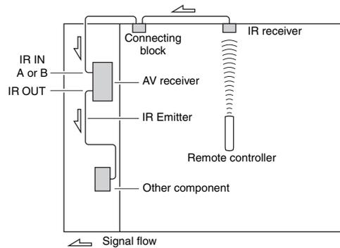
The IR emitter should be connected to the AV receiver's IR OUT jack, as shown below.
