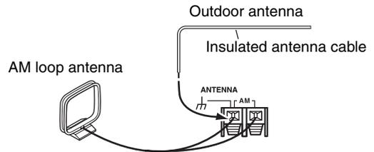
Outdoor AM antennas work best when installed outside horizontally, but good results can sometimes be obtained indoors by mounting horizontally above a window. Note that the AM loop antenna should be left connected. Outdoor antenna must be grounded in accordance with local regulations to prevent electrical shock hazards.
