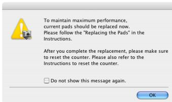
This message only serves as a rough guide for when to replace the feed roller and separation pad. They may wear out sooner if, for example, a lot of paper with rough surfaces is scanned.
