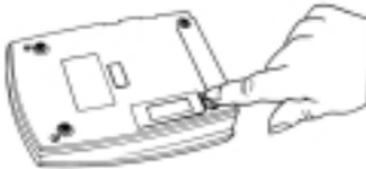
3. Snap the battery's contacts firmly to the battery connector, then place the battery into the compartment.
