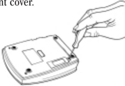
2. Push down the latch to release the battery compartment cover.
