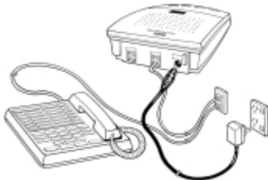
1. Plug the AC Adaptor into the power socket at the rear of the DTAM labelled "9 V AC 400mA".
