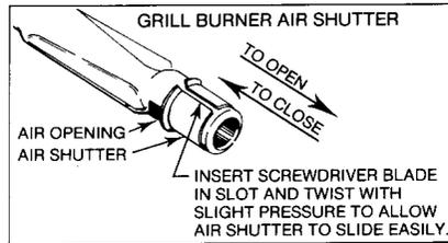
On any burner, closing the air shutter too far will cause the flame to become soft and yellow tipped. Opening the air shutter too wide will cause the flame to blow away from the burner ports. Proper adjustment will produce a sharp, clearly defined, even, blue flame.
