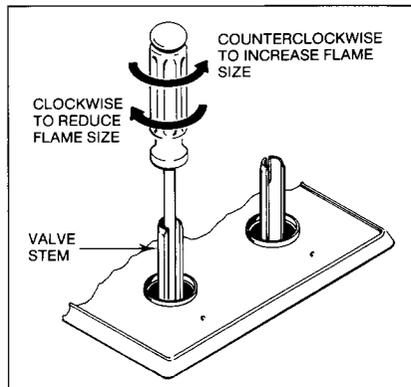
Proper adjustment will produce a stable, steady blue flame of minimum size. The final adjustment should be checked by turning knob from **Hi** to **Lo** several times without extinguishing the flame.
