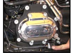
**ST-E:** Position the harness plug for the front pipe under the transmission, along the frame rail. Install the oxygen sensors into the exhaust pipes, connect the harness plugs to the oxygen sensors and secure the harnesses to the frame (above the lowest point) with wire ties.
