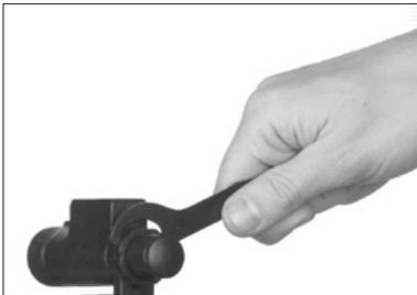
You can also change the position of the IR control panel fitting your needs. Undoing the small set screw on back of IR. Then use the included wrench to loosen back ring, Move the IR to its desired position/angle, retighten ring with wrench then retighten set screw.
