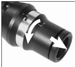
Release detent along arrow "Open" on the sight body, turn it counter clockwise and take it out.
