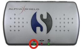
Left LED will turn Green, with the switch at the back of AlphaShield in AUTO/15 Mode (LED will be RED if switch is in LOCK Mode)
