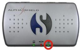
Right LED will turn Green, with the switch at the back of AlphaShield in AUTO/15 Mode (LED will be RED if switch is in LOCK Mode)
