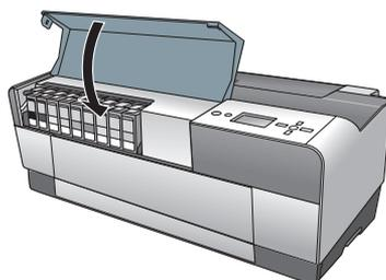
The printer starts charging the ink. This takes 7 or 8 minutes. The LCD displays **READY** when charging is complete.
