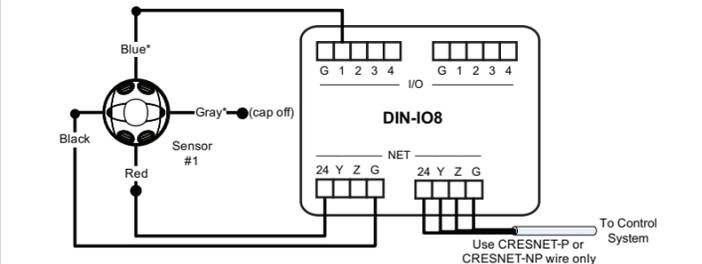
\*\*The following Crestron devices may be used to integrate the sensors into a Cresnet system by following the schematic shown here:
