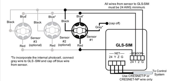
**Connecting Sensors to the DIN-IO8 or Equivalent\*\***
