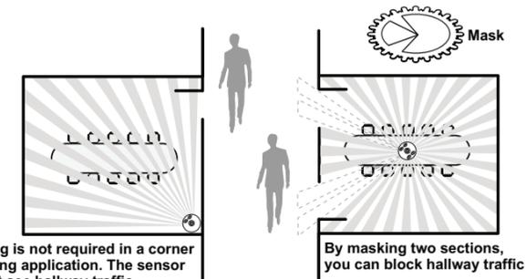
Masking is not required in a corner mounting application. The sensor can not see hallway traffic.
