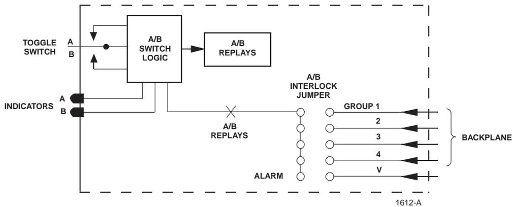
Figure 2-7. Patch Module with A/B Switching Detailed Circuit Diagram
