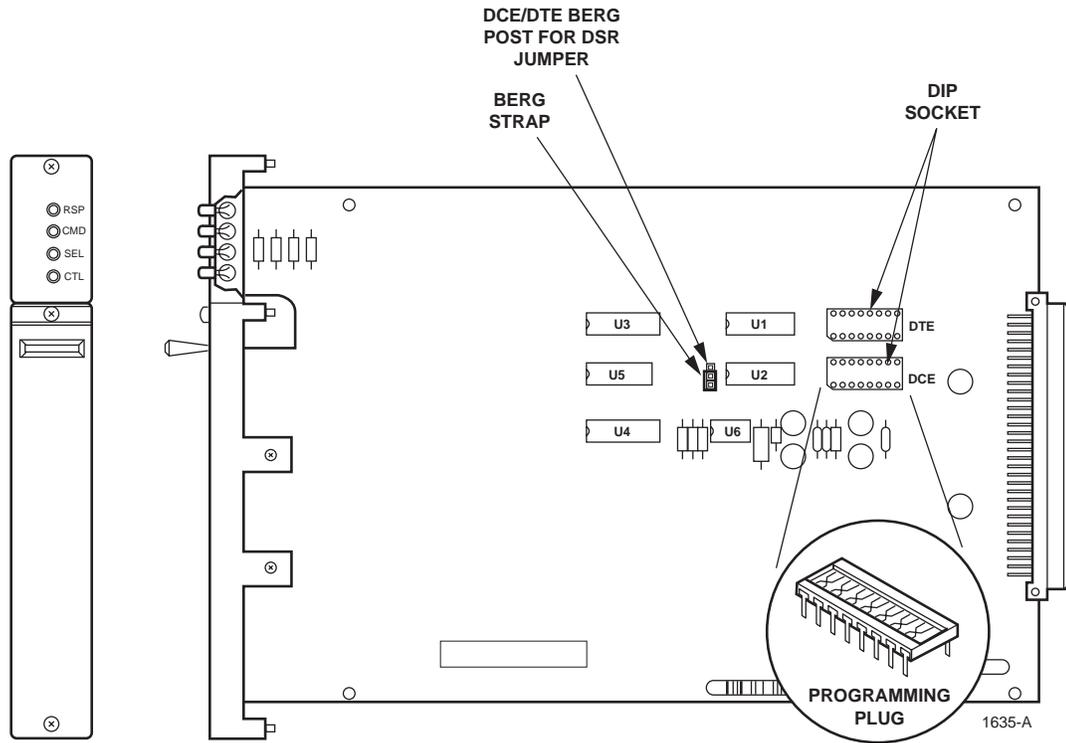
Figure 6-2. Data Converter Module
