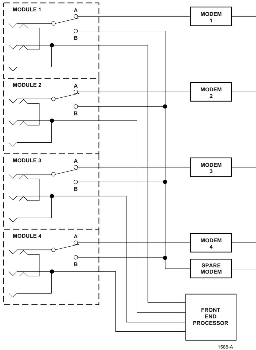
Figure 1-1. Typical Hot Spare Modem Configuration
