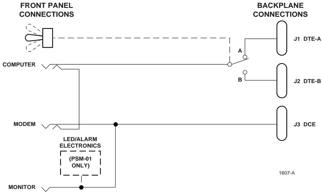
Figure 2-1. PatchSwitch with In-Line Access (PSM-01, PSM-02)
