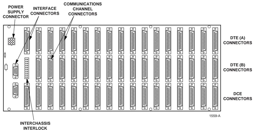
Figure 6-1. RDC-01/02 PatchSwitch Chassis Rear View
