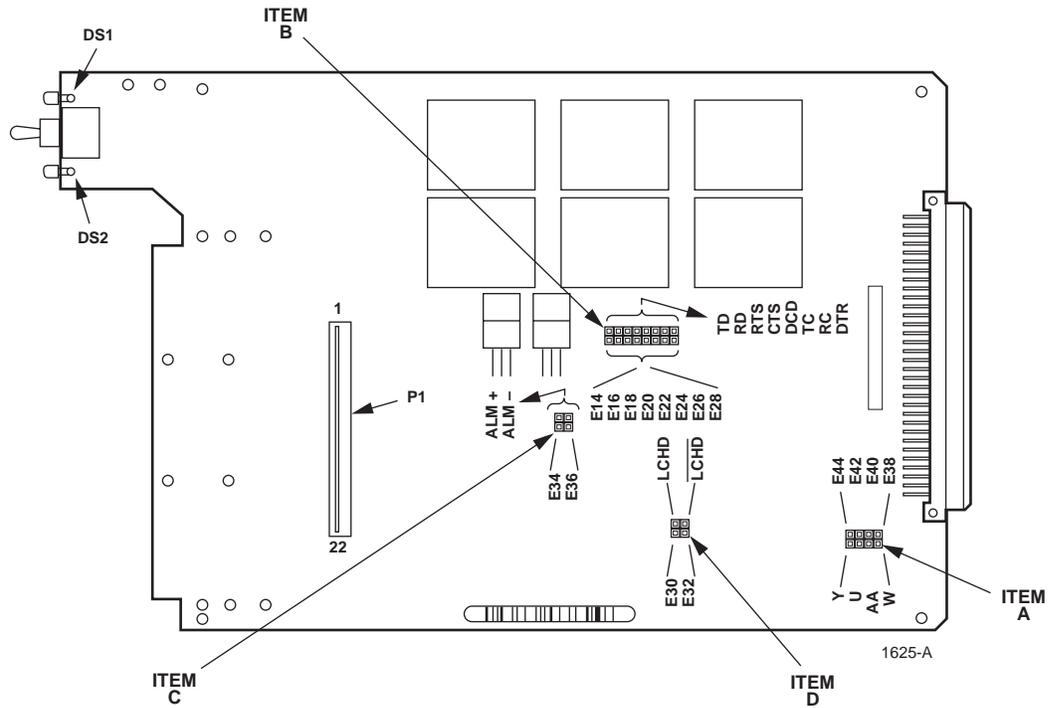
Figure 3-3. PSM-16 and PSM-17 Module PC Board (Component Side)
