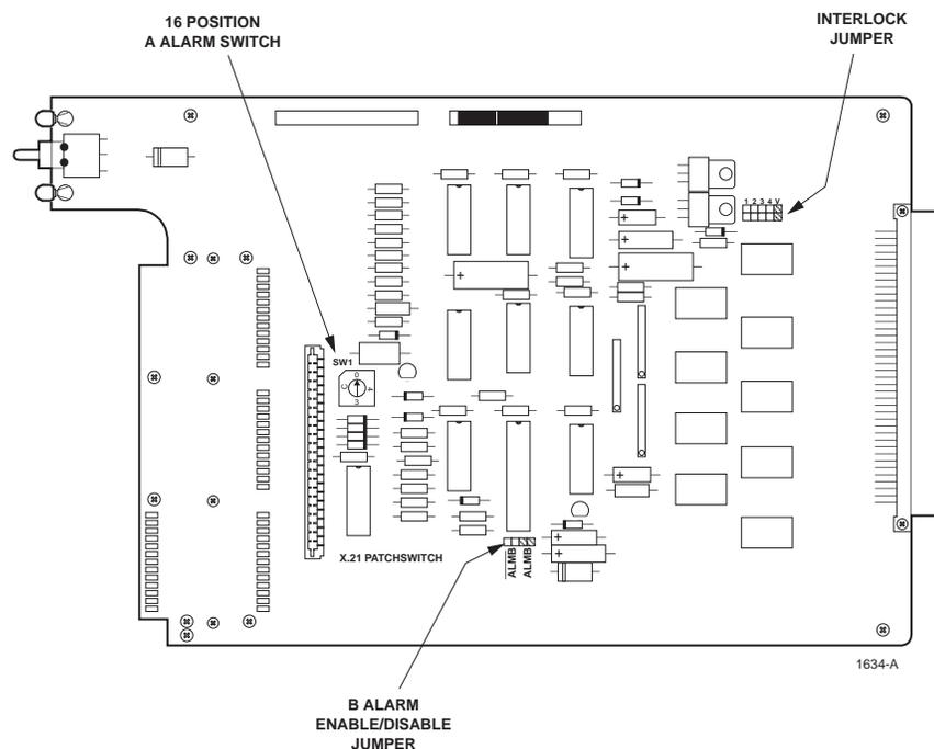
Figure 4-7. Jumper Strap and B Alarm Time Delay Setting Location
