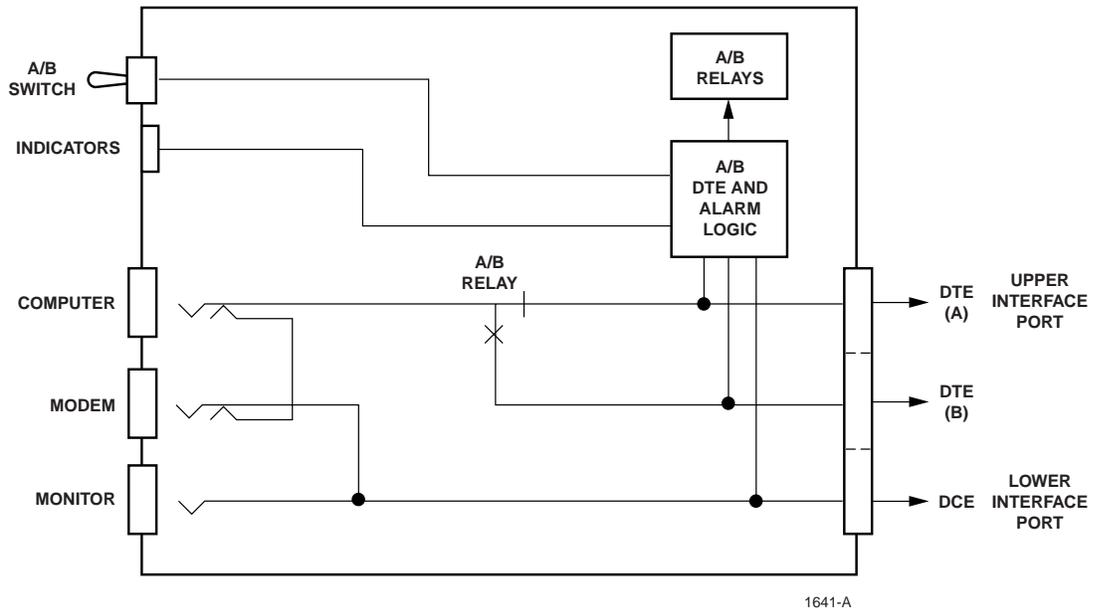
Figure 2-5. LED/Alarm Patch Module with A/B Switching Simplified Circuit Diagram
