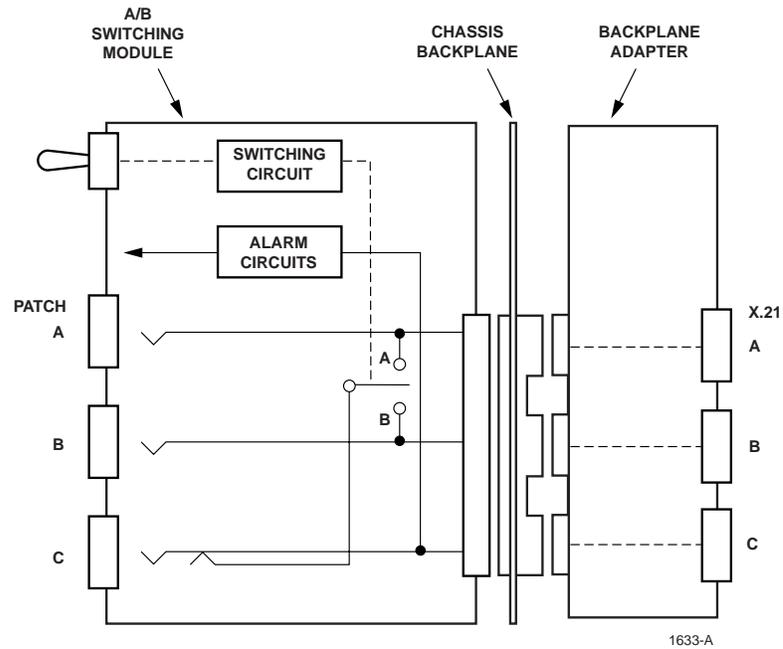
Figure 4-6. A/B Switching Block Diagram
