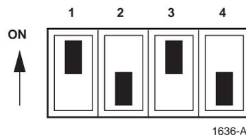
Figure 6-3. Control Module DIP Switch Settings for Chassis 10
