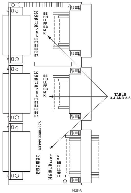
Figure 3-4. FFM-01 and FFM-02 Conversion Board
