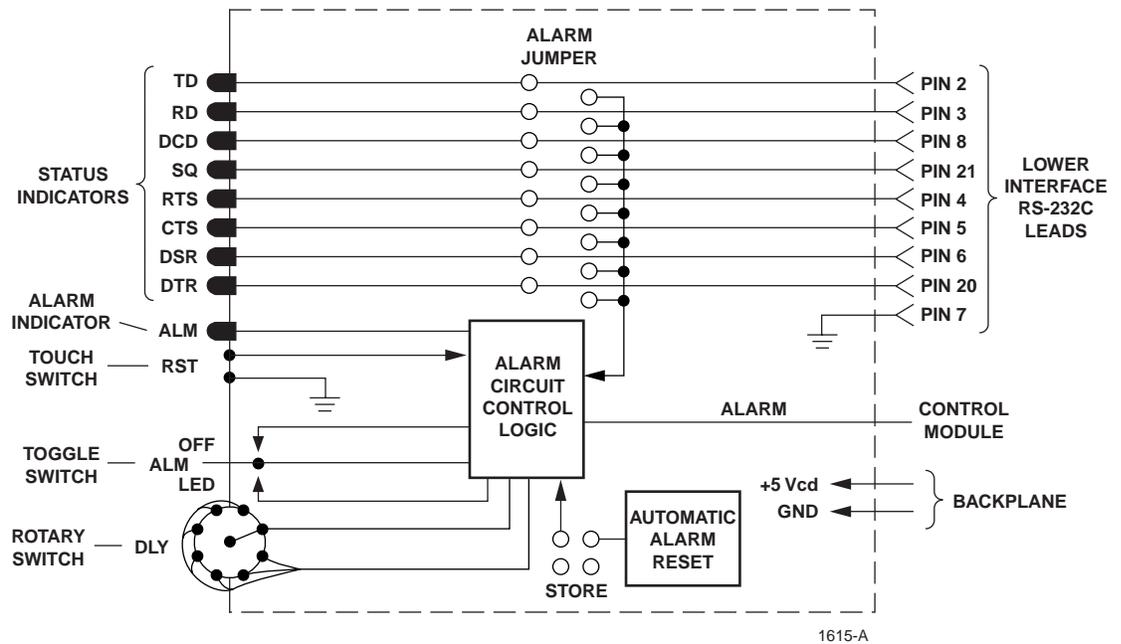
Figure 2-10. LED/Alarm Patch Interface Detailed Circuit Diagram
