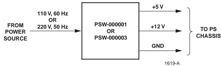
Figure 2-15. PS Chassis Power Supply Block Diagram
