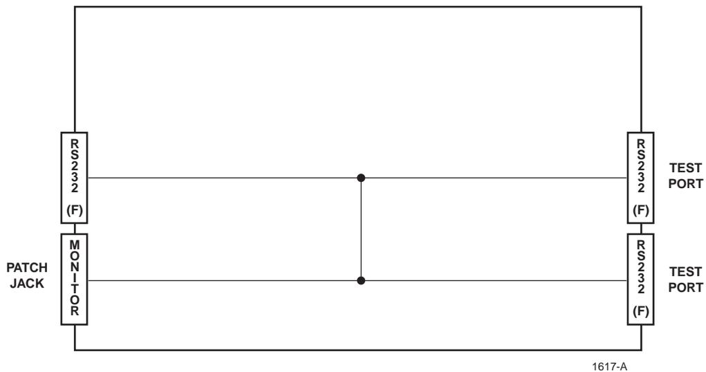
Figure 2-12. PSM-13 Test Module without LED Monitoring
