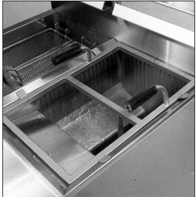
6. After the oil is filtered, close the drain valve and allow the fryer to refill.
