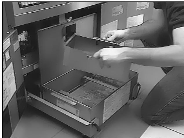
2. Remove the paper hold-down ring (and if changing the filter paper, remove and discard the used filter paper). Remove the filter screen and clean the crumb tray, hold-down ring, filter screen, and pan with a solution of hot water and dishwashing detergent, ensuring that all breadings and food particles are removed from the pan. Ensure the pan is dried completely. Allow the screen to dry completely before reinstalling.
