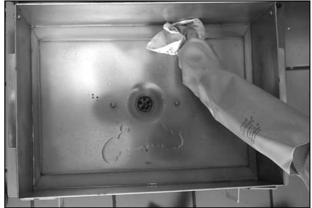
3. After verifying that the metal filter screen is in the bottom of the pan, lay a sheet of filter paper over the top of the pan, overlapping on all sides.
