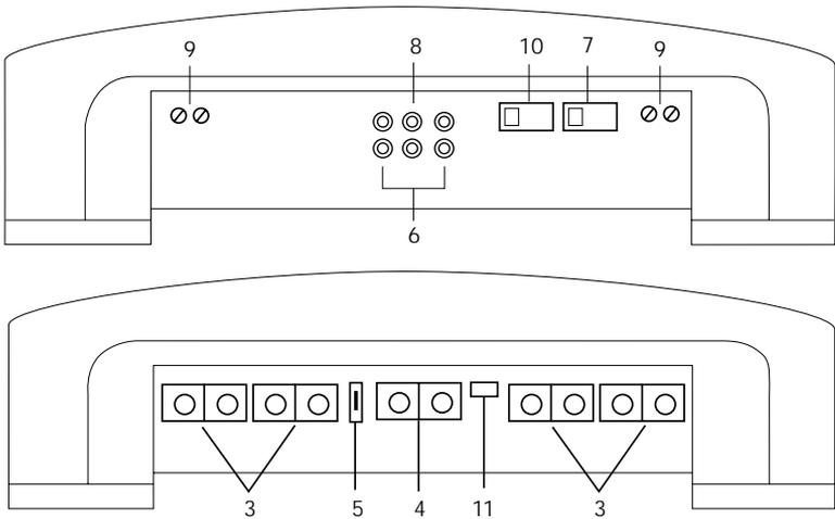
3. **Speaker Terminals** – The heavy duty, gold-plated terminal block connectors (+ and –) will accept wire sizes from 8 AWG to 18 AWG. These gold-plated connectors are immune to corrosion that can cause signal deterioration.
