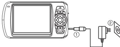
Push the adapter connector into the guide on the right of the network adapter. Push the Network Adapter (2) into a power point that is easily accessible.
