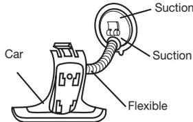
1. Mount the car holder to the flexible neck. Note the labels on the flexible neck. The arrow labeled **CLOSE** must point in the direction of the fixture. The connection closes with a noticeable clicking sound.
