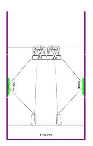
**Front walls**. This loudspeaker is a dipole and therefore there is sound coming from both the front and the back of the speaker. How the front wall (the wall you face while listening) is treated or not treated is important. Generally speaking, the Genesis loudspeakers prefer a live (hard reflective) front wall to a dead (soft absorbent) front wall.
