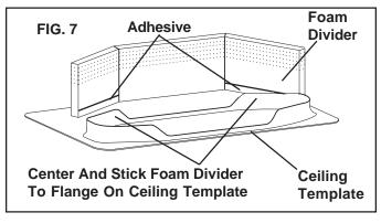
E. Place the ceiling template up into the return air opening in the ceiling. Start each mounting bolt by hand through the ceiling template and up into the base pan. Install a wood screw in each end of the ceiling template. This insures a tight fit of the return air cover to the ceiling. Secure the control box to the ceiling template with thread cutting screw. See figure 8A and 8B.
