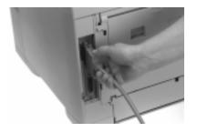
**3** Connect to the computer; tighten the screws.
