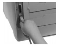
3 Attach to the computer and tighten the screws.
