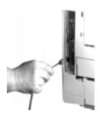
2 Connect the opposite end of the cable into the network.
