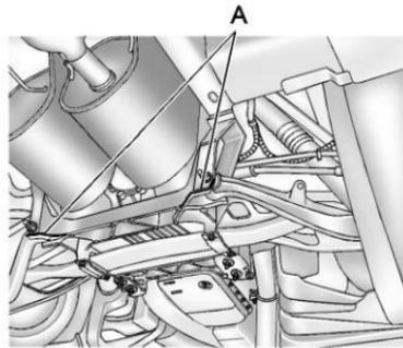
1. Locate the rear lifting points (A), according to the illustration shown.
