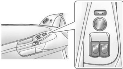
Controls for the outside power mirrors are located on the driver door.
