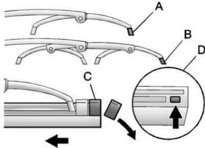
1. Slide the insert (D), notched end last, into the end with the two blade claws (A). Slide the insert all the way through the blade claws at the opposite end (B). The plastic caps (C) will be forced off as the insert is fully installed.
