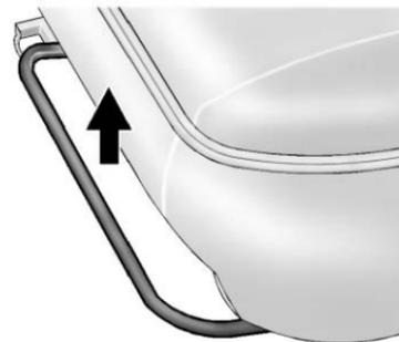
1. Lift the bar under the front edge of the seat cushion to unlock the seat.
