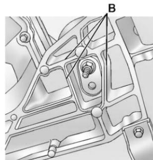
3. Lift the vehicle with the jack, making sure the jack spans at least two of the crossmember ribs (B).
