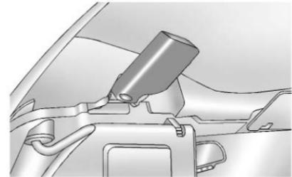
The driver's side handle moves toward the driver's door. The passenger's side handle moves toward the passenger's door.
