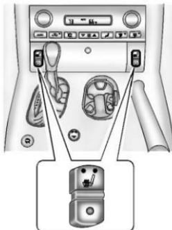
On vehicles with heated seats, the buttons are on the center console. The ignition must be on for this feature to work.
