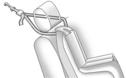
If the position you are using has a fixed headrest or head restraint and you are using a dual tether, route the tether around the headrest or head restraint.
