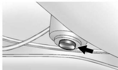
7. Tilt the driver's seatback forward and press the tonneau cover release button located on the underside of the tonneau cover (C) behind the driver's seat. Then raise the tonneau cover (C). If the tonneau cover does not release and three chimes are heard, check to make sure the trunk lid is closed. Also, the cover will not release if the vehicle alarm is armed.
