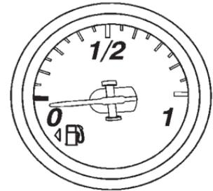
The fuel gauge shows how much fuel the vehicle has left while the engine is on.
