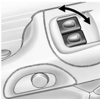
The power window switches are located on each door.
