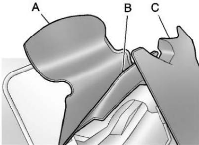
7. Lift the rear edge (B) of the convertible top to its full-up position by first raising the front edge (A).
