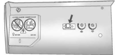
3. Locate in the garage, the garage door opener receiver (motor-head unit). Locate the “Learn” or “Smart” button. It can usually be found where the hanging antenna wire is attached to the motor-head unit and may be a colored button. Press this button. After pressing this button, complete the following steps in less than 30 seconds.
