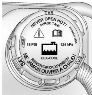
The engine coolant surge tank is located toward the rear of the engine compartment on the driver side of the vehicle. See *Engine Compartment Overview* on page 10-10 for more information on location.
