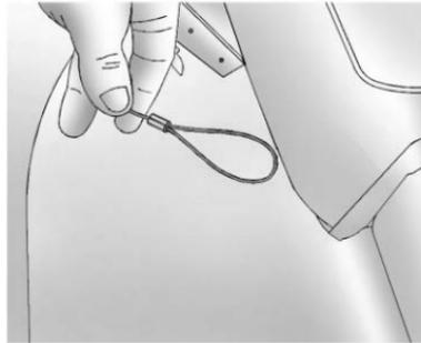
8. Pull the cable to release the tonneau cover.
