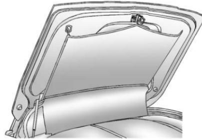
3. Grasp the loop at the rear center of the shade and wrap it around the striker assembly.
