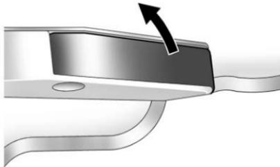
1. From inside the vehicle, use the door release handle located on the floor next to each seat. Pull the handle up to unlock and unlatch the door.
