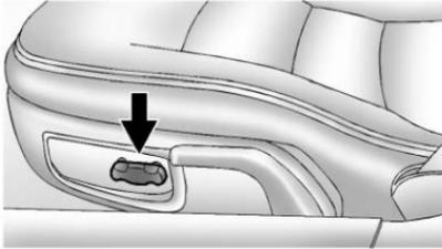
On vehicles with power seats, the control is on the outboard side of the seat.
