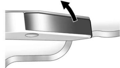
Pull the door release handle located on the floor next to the seat.
