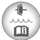
The hydraulic clutch fluid reservoir cap has this symbol on it. See *Engine Compartment Overview* on page 10-10 for reservoir location.
