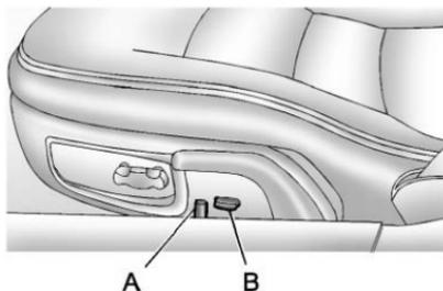
On vehicles with power lumbar and side bolsters, the controls are on the outboard side of the seat.
