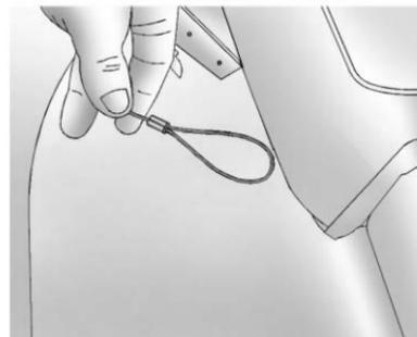
1. Open the tonneau cover by pulling the emergency release cable.
