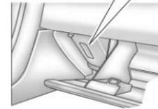
7. Place the new transmitter in the glove box transmitter pocket with the buttons facing the passenger side.
