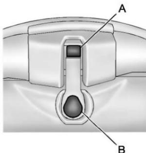
7. To unlock the rear of the roof panel's rear release latch, press the back of the release handle (B). Then press the button on the front of the release handle (A).
