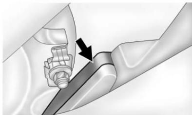
The ZR1 also has an electronic brake pad wear sensor system. When pads are worn, the CHANGE BRAKE PADS message displays in the Driver Information Center. See *Brake System Messages* on page 5-36.
