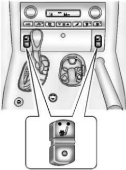
On vehicles with heated seats, the buttons are on the center console.
