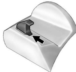
2. Insert the roof panel so that the outside front edges line up between the receiver covers. Push forward on the roof panel until it stops.
