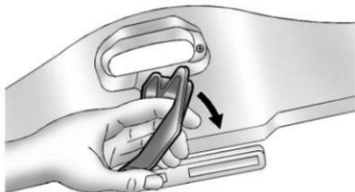
4. The convertible top front latch, located above the inside rearview mirror, must be unlocked. Pull the convertible top front latch down and turn it clockwise to unlock it.
