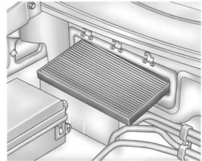
3. Remove the filter and install the new air filter.
