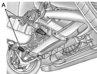
1. Locate the front lifting points (A), according to the illustration shown.
