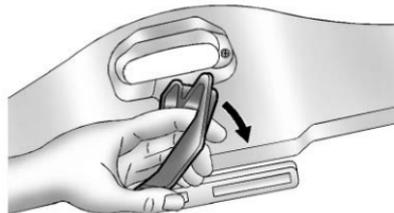
3. Release the convertible top front latch, located above the inside rearview mirror, by pulling and turning it clockwise toward the driver's door. Push upward on the front edge. The windows will automatically lower.
