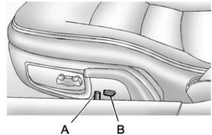
On vehicles with power lumbar and side bolsters, the controls are located on the outboard side of the seat.
