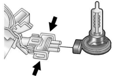
4. Remove the headlamp bulb by releasing the outer tabs from the socket.
