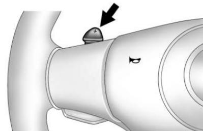
The Manual Paddle Shift system is activated from S (Sport Mode) by pushing the paddle, above the steering wheel spokes, to up-shift to the next gear, or pulling on the paddle, behind the steering wheel spokes, to down-shift to the next gear.
