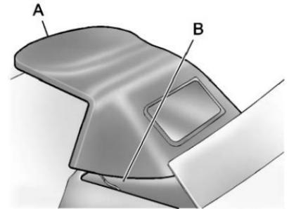
9. Push forward on the front edge (A) of the convertible top to allow the rear edge (B) of the convertible top to be moved to its full-down position.
