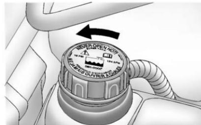
1. When the cooling system, including the coolant surge tank pressure cap and upper radiator hose, is no longer hot, remove the pressure cap.
