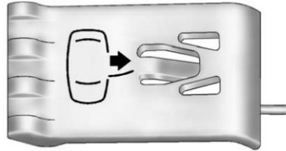
2. From outside the vehicle, use the key in the cylinder above the license plate to open the hatch. Then, use the door release tab (A), located on the carpet inside the hatch on the driver's side of the vehicle. Pull the tab to unlock and unlatch the driver's door. See *Keys* on page 2-2 for information on opening the hatch during a loss of power.
