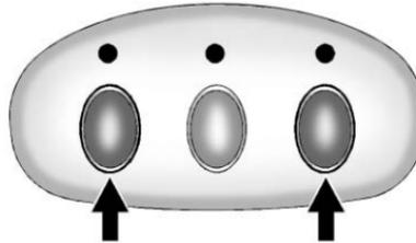
2. From inside the vehicle, press the two outside buttons at the same time for one to two seconds, and immediately release them.
