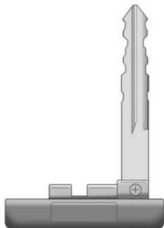
The key, located inside the keyless access transmitter, can be used to lock and unlock the glove box and
