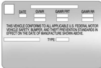
A vehicle specific Certification label is attached to the rear edge of the driver's door.
