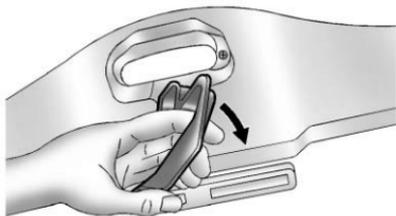
5. Pull the convertible front top latch down and turn it counterclockwise to lock the convertible top.
