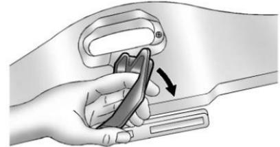
11. Pull the top front latch handle down and turn it counterclockwise to lock the convertible top.
