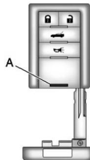
Press the button (A) near the bottom of the keyless access transmitter to remove the key. Never pull the key out without pressing the button.
