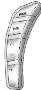
The HUD controls are located to the left of the steering wheel.
