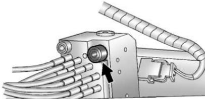
3. Locate the pressure release bolt on the front side of the hydraulic pump.
