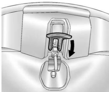
6. Turn the front release handles inward so that they latch to the closed position.
