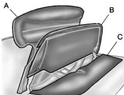
5. Lift upward on the front edge (A) of the convertible top off of the windshield frame. Then lift upward on the rear edge (B) of the convertible top so it is vertical to the tonneau cover (C). The front edge (A) and rear edge (B) should be straight up.
