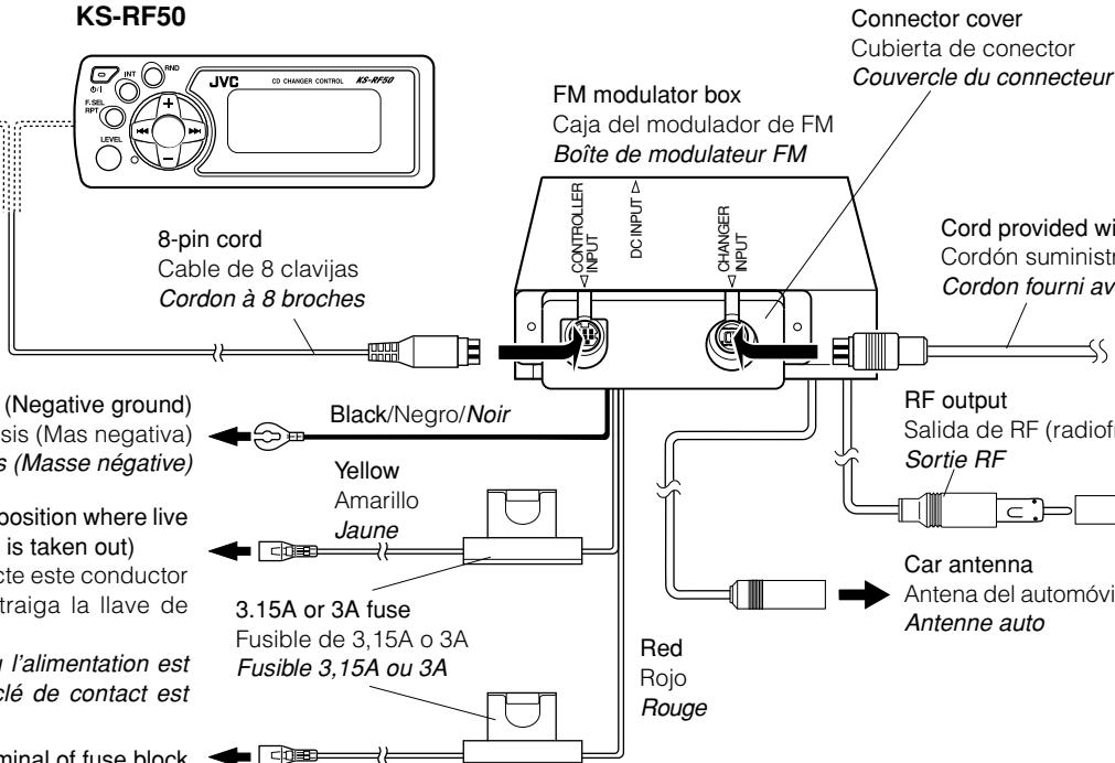
When you use the connector illustrated on the left, remove the connector cover (see "How to disconnect the cords," step 1.)
