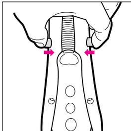
Press Handheld release buttons inward to release Handheld unit.
