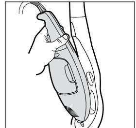
Remove Handheld unit from floor unit. DO NOT pull power cord when removing
