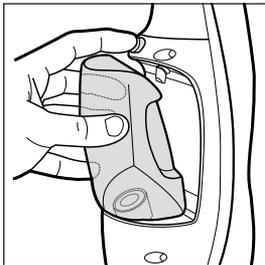
Press Water Tank Release button and remove water tank.
