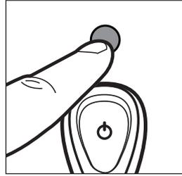
To use steam control, hold in steam control button to engage the lower steam setting.
