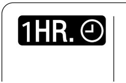
This function causes the unit to operate for one hour and then stop, regardless of whether the unit is on or off when this button is pressed. The **1HR. ⏰** indicator in the display indicates that this function is operating.
