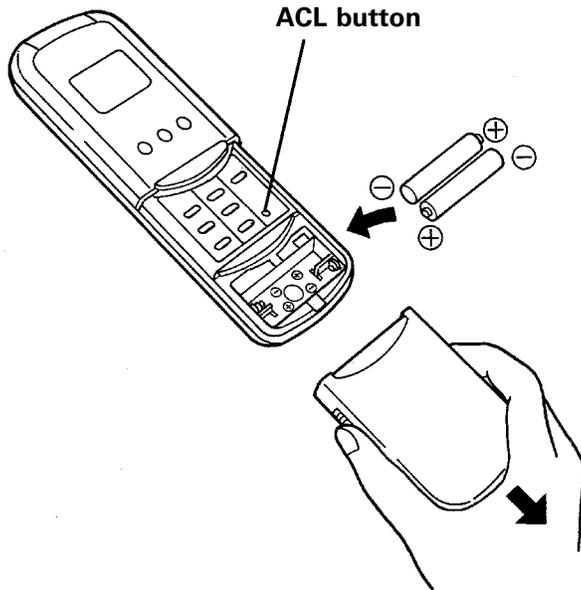
1. Slide the cover in the direction indicated by the arrow and remove it.
