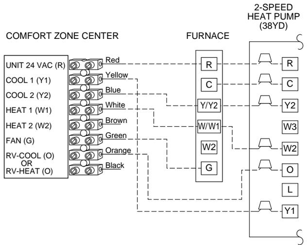
**NOTE:** 38YD – with dual fuel, use the 38YD “Furnace Interface” and “Balance Point” feature on the heat pump control to operate dual fuel option. Configure the 4-Zone controller to act as if it were controlling a single speed heat pump. Turn (T-6) ON. Turn (T-9 & T-26) OFF. Set (S-7) to 0. (Let the 38YD perform the dual fuel optimization).
