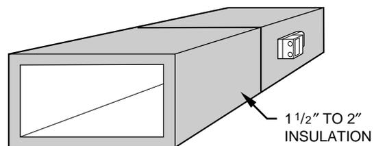
**Fig. 15—Insulated Rectangular Fibrous Glass Duct Work** A95134
