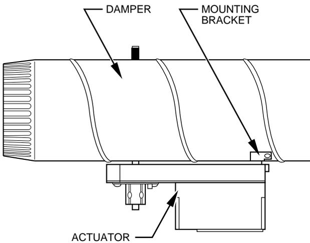
**Fig. 6—Damper Motor Positioning** A95128
