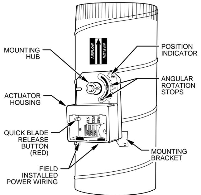
**Fig. 7—Damper 24-vac Connections** A95096
