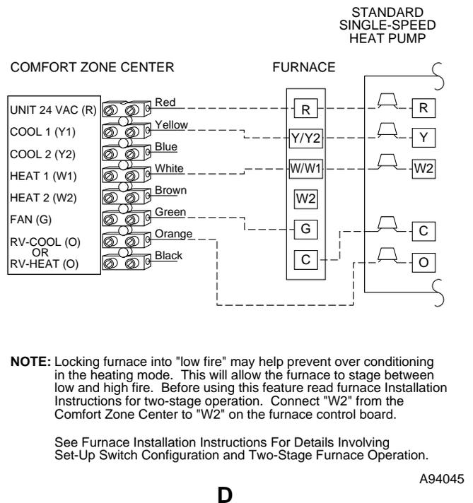
**Fig. 22—Typical Wiring Diagram (Furnace with Heat Pump)**
