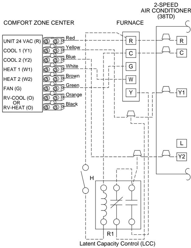
R1 = Relay DPST, Pilot Duty, 24-v coil (HN61KK324) or Equivalent.
