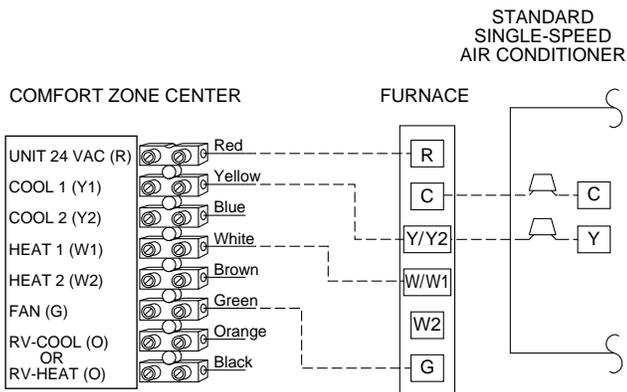
**NOTE:** Locking furnace into "low fire" may help prevent over conditioning in the heating mode. This will allow the furnace to stage between low and high fire. Before using this feature read furnace Installation Instructions for two-stage operation. Connect "W2" from the Comfort Zone Center to "W2" on the furnace control board.
