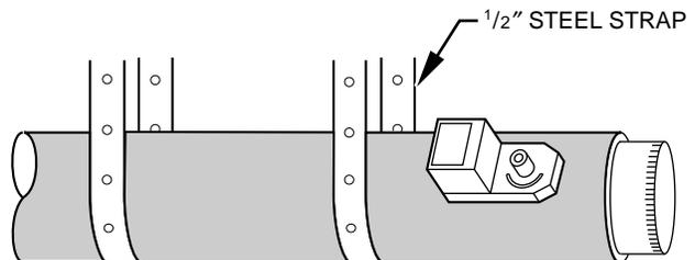
**Fig. 9—Insulated Round Metal Duct Work** A95130
