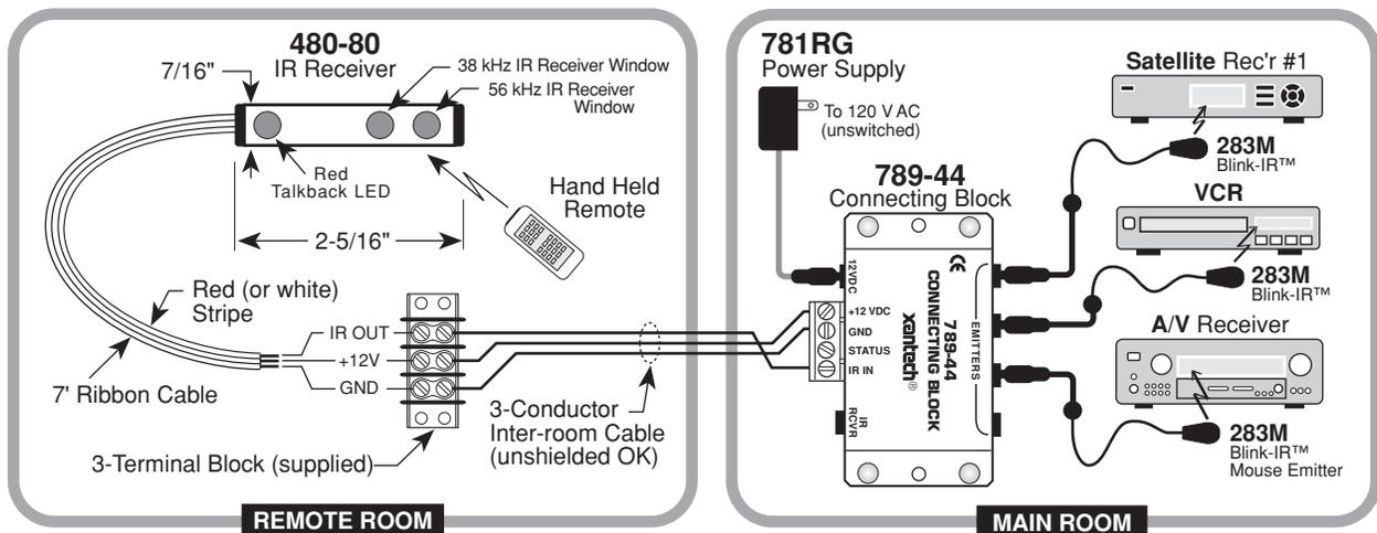
Fig. 1 A 480-80 in a basic IR repeater system.
