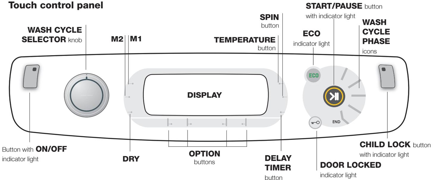
Button with **ON/OFF** indicator light: press this briefly to switch the machine on or off. The green indicator light indicates that the machine is switched on. To switch off the washer-dryer during the wash cycle, press and hold the button for approximately 3 seconds; if the button is pressed briefly or accidentally the machine will not switch off. If the machine is switched off during a wash cycle, this wash cycle will be cancelled.
