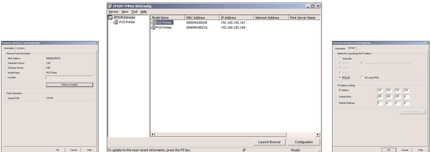
Epson's Ethernet module offers a simple, intuitive Microsoft® Windows® utility for configuring your Epson printers for network operation.
