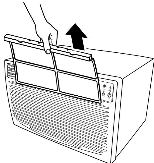
3. Use a vacuum cleaner to clean air filter. If air filter is very dirty, wash it in warm water with mild detergent. Do not wash air filter in the dishwasher or use any chemical cleaners.
