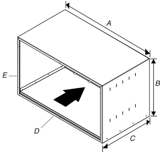
A. Width (W)      D. Horizontal insulation strip
