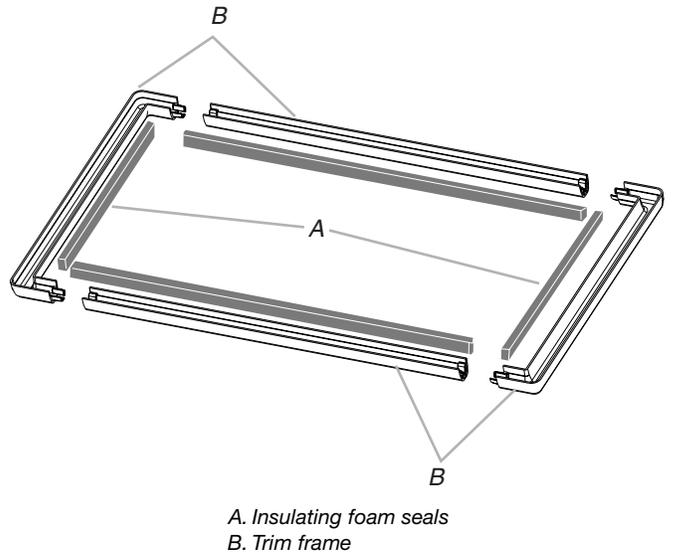
3. Slide the trim frame onto the air conditioner until the foam makes a seal with the wall sleeve.
