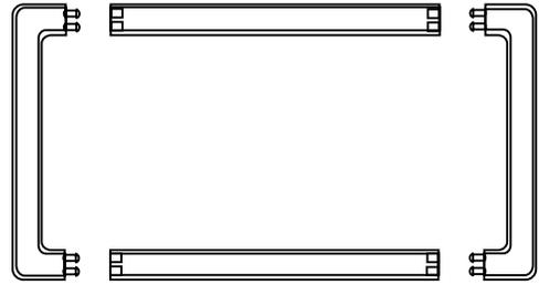
2. Install the 1/8" insulating foam around the inside edge of the trim frame. Begin in the bottom left corner and place the insulating foam around the entire inside of trim frame. Check to be sure foam is flush with the bottom edge of the trim frame.
