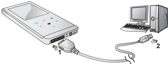
1. Connect the larger end of the USB cable to the USB Connection Port on the bottom of the player.
