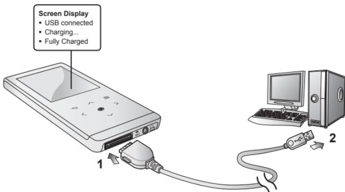
1. Connect the larger end of the USB cable to the USB Connection Port on the bottom of the player.
