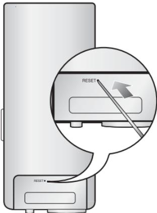
Press the Reset hole at the rear of the player with a pointed object such as a safety clip.
