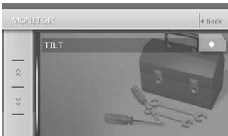
3. Repeat touching the [O] key to adjust the angle of the liquid crystal panel. Every touching the [O] key tilts the liquid crystal panel forward or backward. The adjusted angle is stored in memory.
