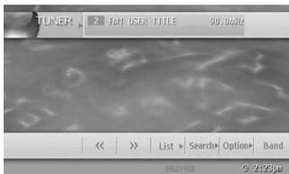
2. Press the [BAND] button or touch the [Band] key to select the radio band. Each time the button is pressed, the radio reception band changes in the following order:
