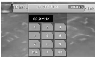
3. Touch the [0]~[9] key corresponding with the frequency you desired. When you input the wrong number, touch the [CLR] key to delete the last input number.
