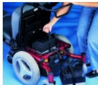
*The individual batteries can easily be lifted out of the base, using straps.*
