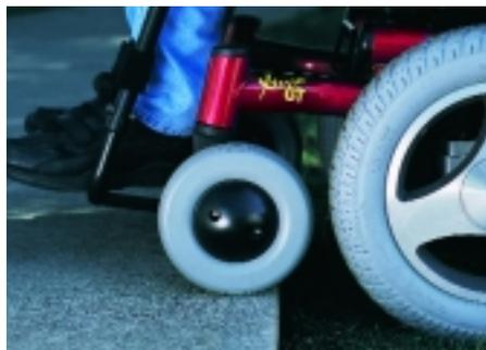
*Weight is transferred to the drive wheels, providing both traction and motor strength to elegantly pull the user and chair over the obstacle.*
