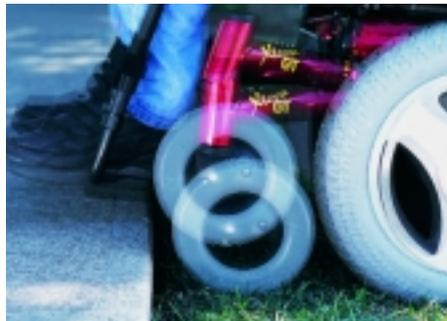
*The high torque of the new motors lifts the front wheels to facilitate the change in pitch.*
