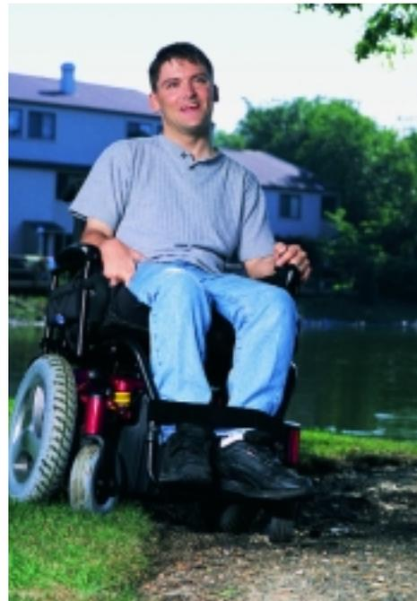
*The six wheels of the GT remain in contact with the ground for maximum stability, safety and traction when negotiating uneven terrain.*
