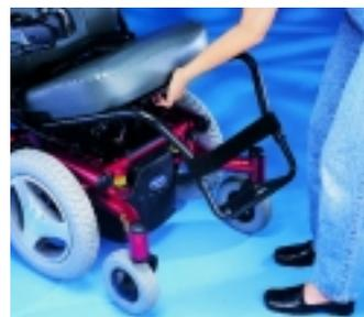
*By releasing the latch under the seat, the GT seat frame pivots rearward, allowing access to the 22NF batteries.*
